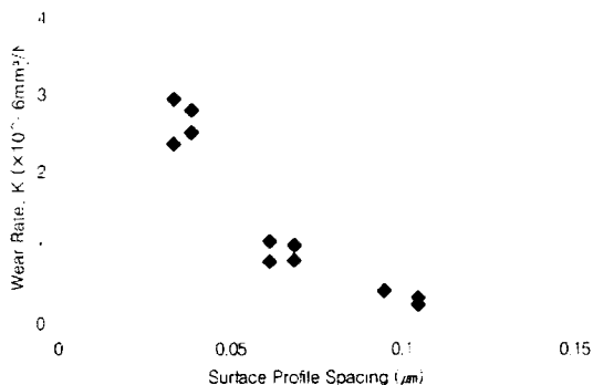
Fig. 6 Effect of surface profile spacing on the wear rate
